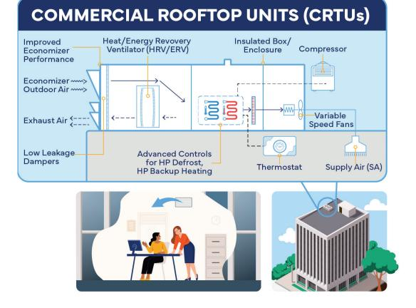
The CalMTA team is conducting energy modeling and testing to understand the energy efficiency and decarbonization opportunities specific to California climate zones. This work will assess equipment performance, the benefits of recovery systems, component sizing, emission impacts, and lifecycle testing.
