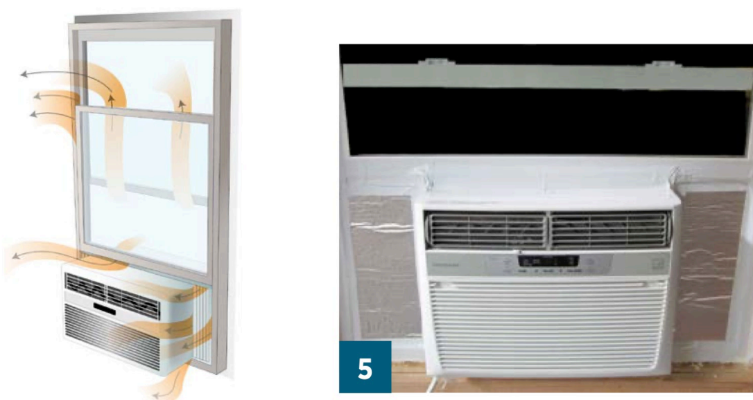
Figure 11. Left: Common air infiltration pathways for window heat pumps. Right: Proposed energy efficient sealing by NREL.
